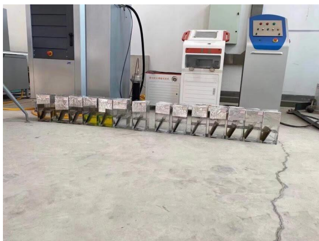
Immersion experiments were conducted on membrane materials in 14 different media at Sinopec Institute of Safety.
